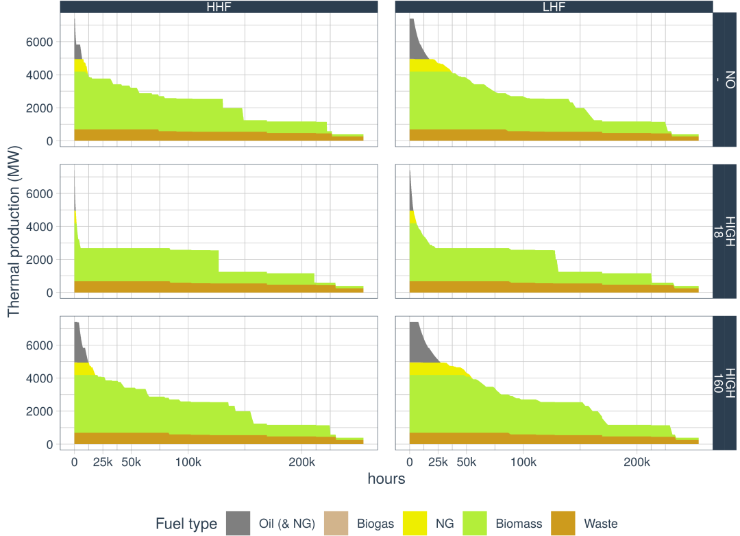
Figure 6: Resulting thermal power load duration curves, per production type (aggregated), on hourly basis over all 29 years. Top: NO hydrogen scenario, middle: HIGH hydrogen at a value of 18 \text{ € MWh}^{-1} , bottom: HIGH hydrogen at a value of 160 \text{ € MWh}^{-1} . Left: HHF, right: LHF.
