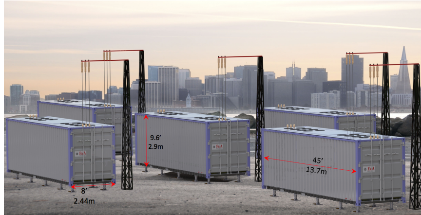
Figure 7: 5x Clustered Holos Quad generators, 65 MWe total generation Each generator is positioned to ensure adequate passive air-flow, external shields not shown
