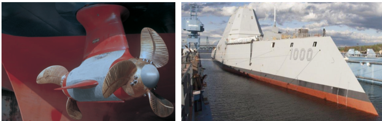
Figure 29: (left) Electric propulsor, (right) USS Zumwalt (DDG 1000) with Integral Electric Propulsion (IEP)
