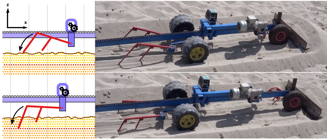
Figure 3: Push-pull bulldozer with interlocking spikes. Motion is from left to right.
