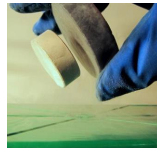
Figure 1: Cryocooled superconductor with a pinned permanent magnet suspended in gravity
