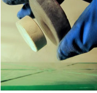
Fig. 1. Cryocooled superconductor with a pinned permanent magnet suspended in gravity.
