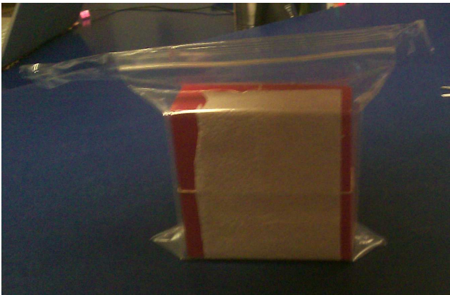
Figure 3: This figure shows the process of sealing a cryobox with absorbent paper into a plastic bag.
