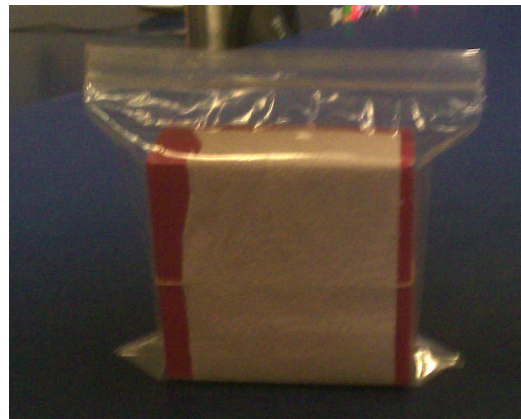
Figure 3: This figure shows the process of sealing a cryobox with absorbent paper into a plastic bag.
