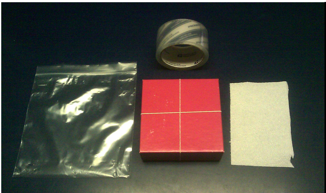
Figure 2: Supplies for sealing a cryobox inside a plastic bag. (Each cryobox needs its own plastic bag and piece of absorbent paper.)
