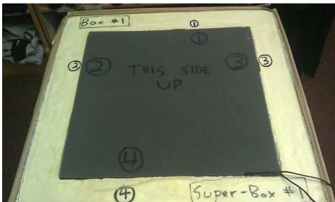
Figure 7: This photograph shows the appearance of the top of the super-box with the foam lid in place. The black wires lead to thermometer probes.
