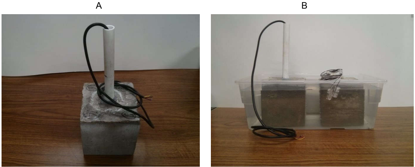
Figure 4: A) Final temperature/humidity sensor assembly and B) soaked sensors
