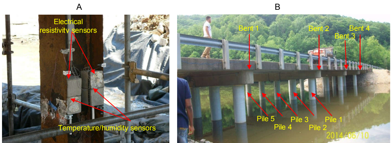
Figure 11: A) Electrical resistivity and temperature/humidity sensors installed in the field and B) East Lynn Lake Bridge after rehabilitation, showing pile identification labels
