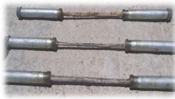
Figure 1 HFRP reinforcements with end anchorages for tensile tests
