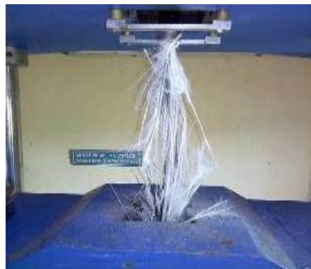
Figure 2 Failure of HFRP reinforcements tensile test
