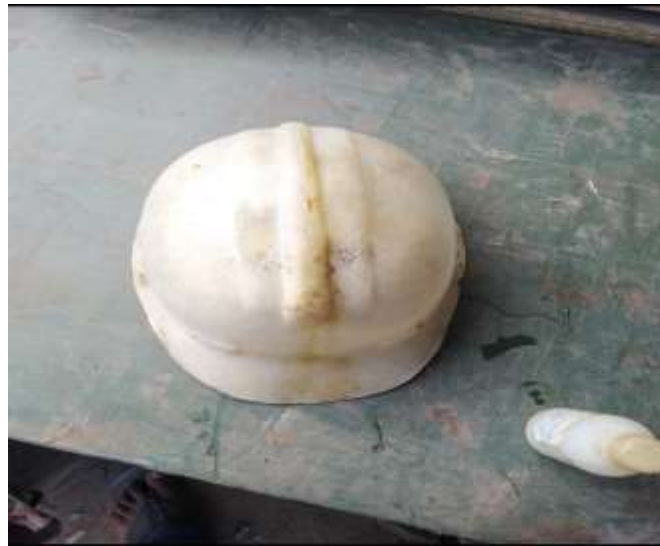
Figure 3 Fabricated Industrial Safety Helmet
