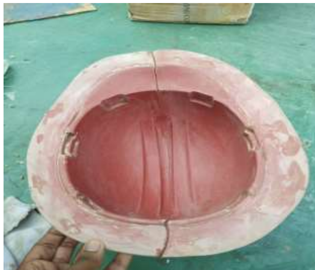
Figure 2 Mould cavity for Safety helmet
