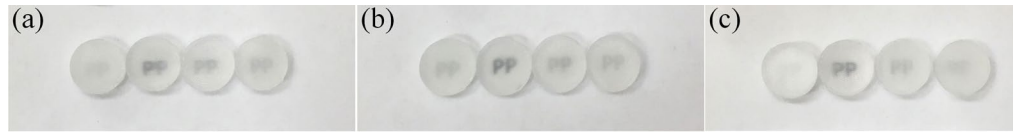
Fig. 2. (a) Slices printed with different infill flow rates (increase from right to left). (b) Slices printed with different infill speeds (decrease from right to left). (c) Slices printed with different layer heights (decrease from right to left)
