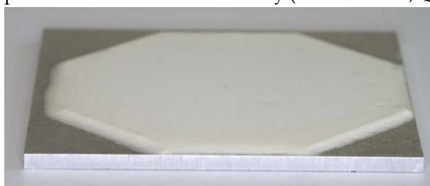
Figure 2: Sample Ct_610 with 0.61 mm coating thickness
