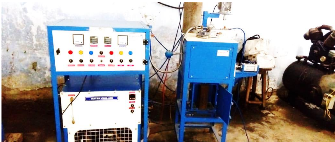
Figure 1 Experimental setup for fabricating Al7075 and B 4 C particles.
